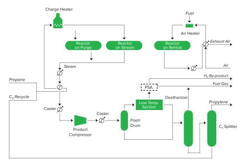
The diagram shown is for the production of propylene. A deoiler is also included to reject a small amount of  $C_4$ s and heavier material. For isobutylene production, the deethanizer and  $C_3$  splitter are replaced by a depropanizer. For n-butane to n-butenes, the reactor effluent is cooled by a quench oil system and n-butane is recycled from the downstream alkylation unit.
