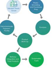
A key piece of the energy transition is the circular economy. In the circular economy of our industry, Lummus licenses a leading plastic waste conversion technology based on thermal pyrolysis that will help reduce plastic waste through integrated processing solutions for turning end-of-life plastics into pyrolysis oil. This pyrolysis oil can then be processed back into plastics or blended into fuels.
